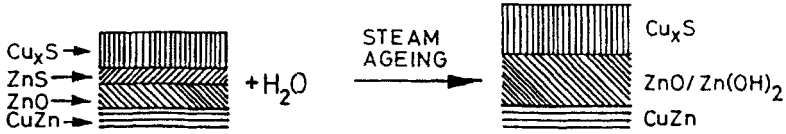
FIGURE 7 Schematic presentation of interfacial film formed between rubber and brass due to steam ageing.
